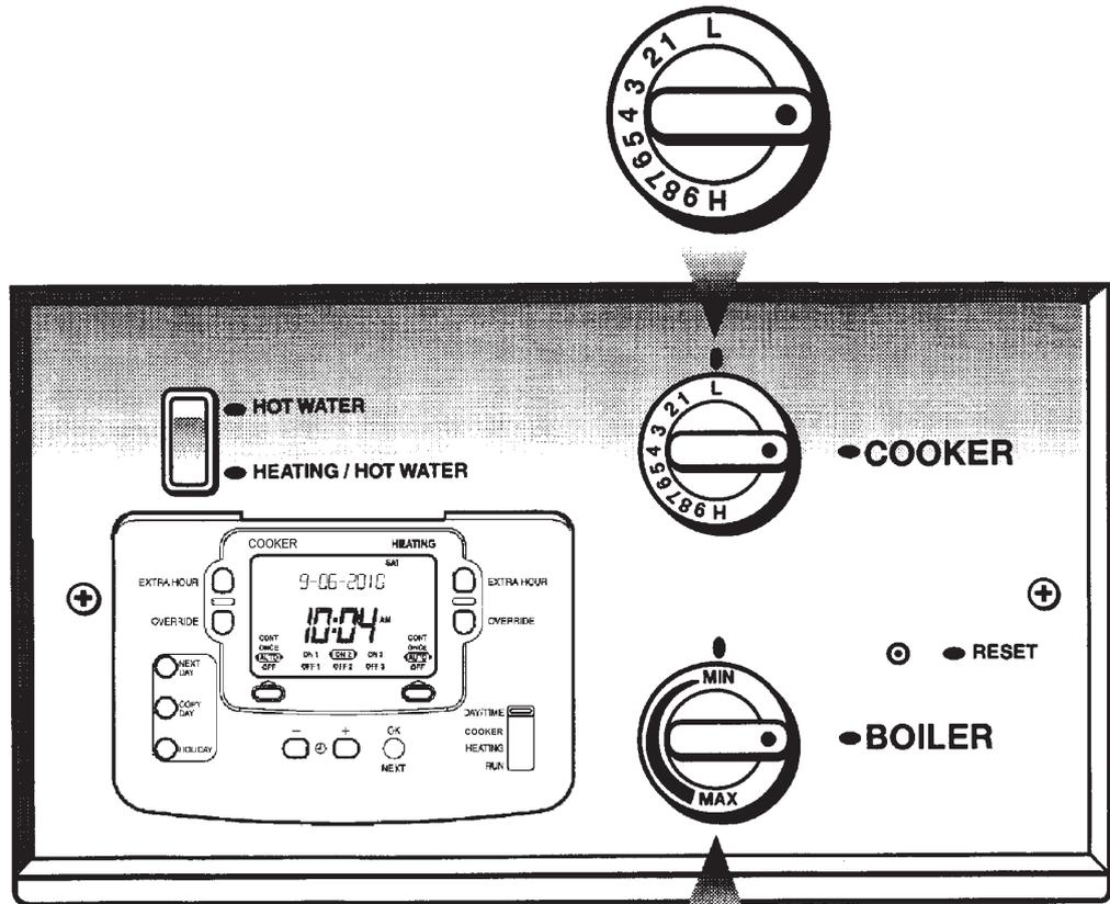
When the cooker control knob is in the vertical park position, the cooker burner may come on if the temperature in the oven is cold enough until the temperature reaches approximately 25°C. To overcome this it is recommended that 'cooker off' is selected on the programmer when not in use.
